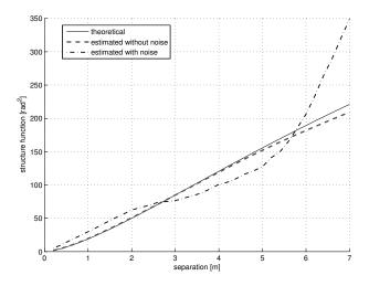
Fig. 2. In solid line the theoretical structure function, with  $L_0 = 50$ m and  $r_0 = 0.4$ m, as a function of space distance. In dashed line the structure function values estimated from noise-free samples. In dashed-dotted line the structure function values estimated from noisy SH measurements.
