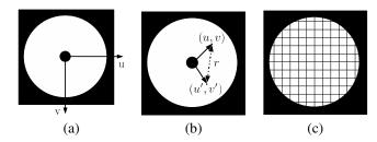
Fig. 1. (a) Coordinates on the telescope image domain. (b) Two points, (u, v) and (u', v'), separated by a distance r on the telescope aperture plane. (c) Discrete domain  $\mathbb{L}$ .
